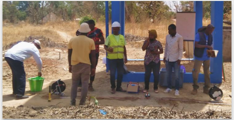
Team executing resistivity siting measurements
