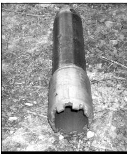
Figure 2 Hammer head or bit
