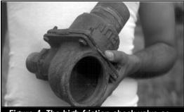
Figure 4 The high-friction check valve as used on shallow tube wells
