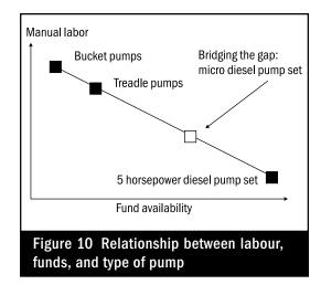
Diesel pump sets (5 hp [horsepower]), fitted on a tube well or dug well are the next best, but funds will be a major constraint for many. There seems to be a niche for small-hp micro diesel pump sets (Figure 10).
