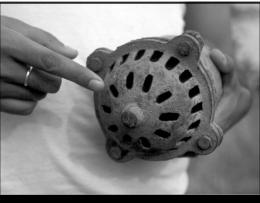
Figure 6 The high-friction foot valve as used on dug wells or pumping from surface water
