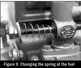
Figure 9 Changing the spring at the fuel pump for reducing the engine speed
