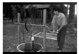
Figure 8 Rope pump installed on a dug well
