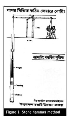
to be hollow with steel<sup>1</sup> teeth welded to its side, so that it can collect the crushed material and soil particles. The pipe and the hammerhead need to be raised repeatedly to remove the material collected in the bit. To minimize the chances of material falling out 0.6–0.8 m have to be hammered at a time, so that the soil and stone particles remain firmly compacted inside the bit.
