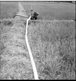
Figure 2 Lay-flat hose used with diesel pumpset
