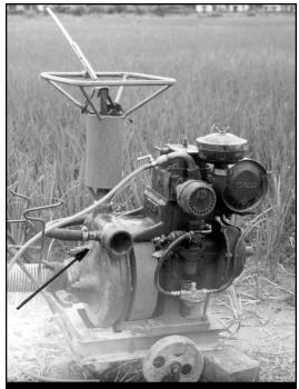
Figure 11 Half-pipe for creating cooling water flow pressure
