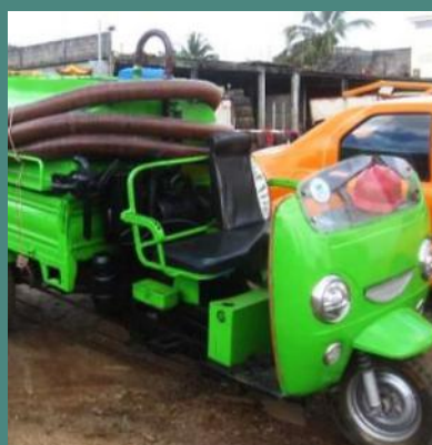
Fig.2 Sludge removal tricycle (750 liters)
