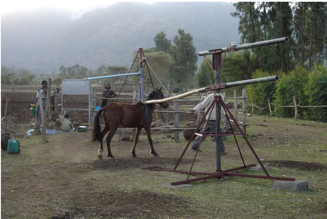
foto: Testing animal driven pump in the vicinity of Butajira
