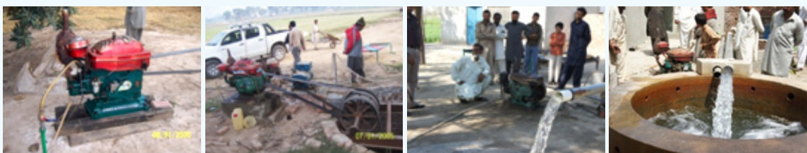
Photos clockwise: Petter engine, engine and fan belt assembly, engine drawing water
