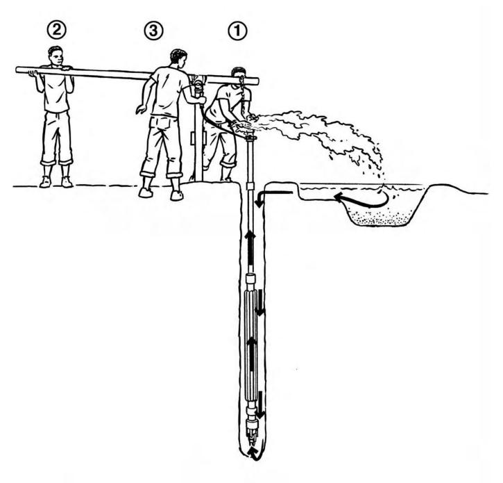
Fill the drill pipe with water Pour water into the drill pipe until it is filled and close the pipe quickly with your hand. Now sludging can begin.
