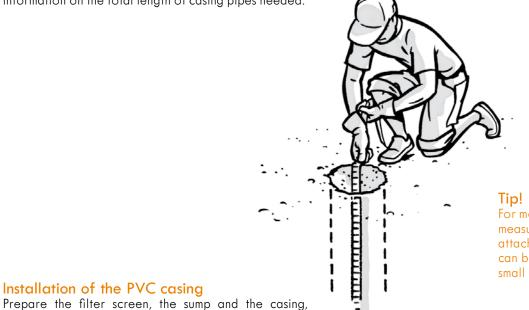
Tip! For measuring; use a rope or long measuring tape with a small weight attached. Measuring with a rope can be best done when you make small knots at every meter.
