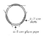
cutting and bending the bottom of the PVC pipe.
