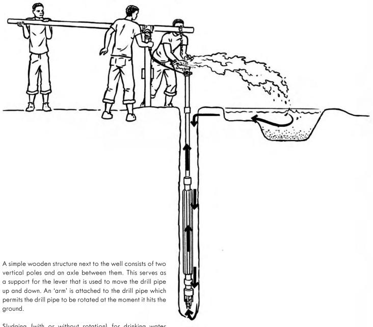
Sludging (with or without rotation) for drinking water wells is generally used up to depths of about 35 meters on average, and exceptionally deeper in soft formations.
