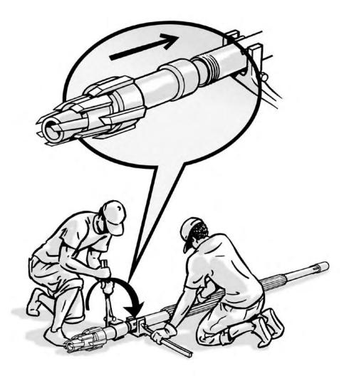
Tip Keep threads clean with a steel brush and protect threads during transport to prevent damage.
