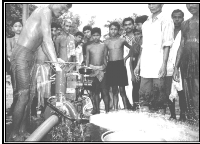
Figure 5.1; testing of a pumpset after maintenance
