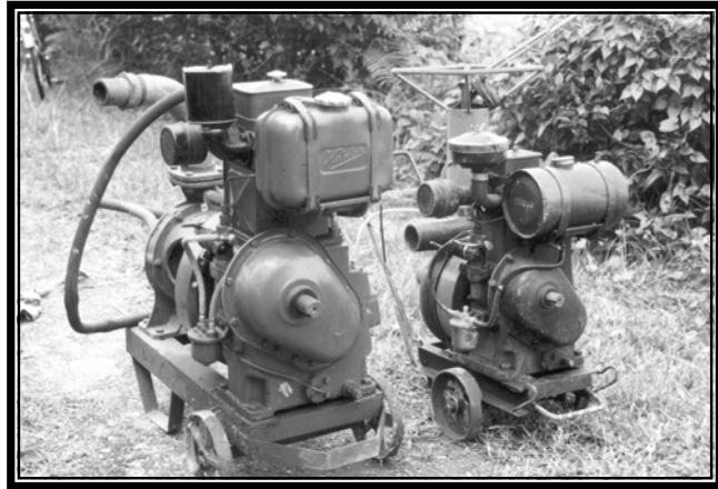
Figure 7.1; standard 5hp pumpset (left) and the new model 2.5hp pumpset (right)
