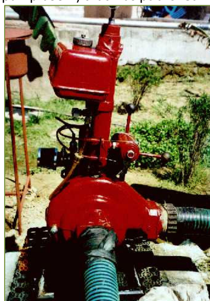
Figure 3; early proof-of-concept of the Lohmann micro diesel pump
