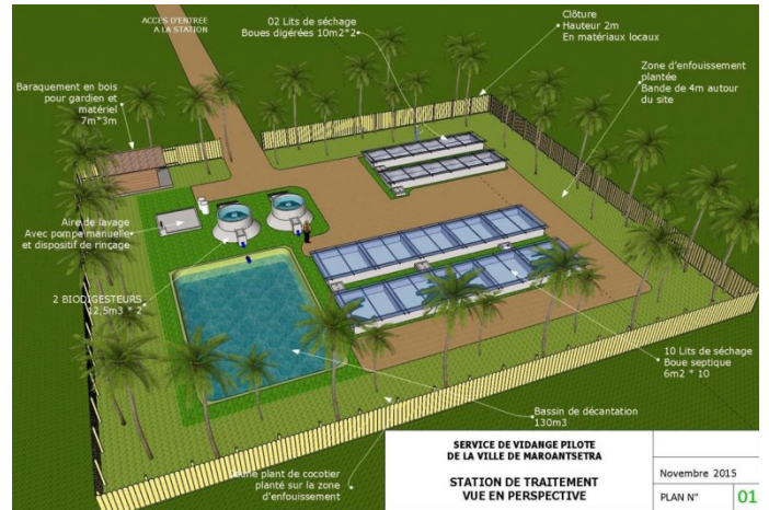
Fig.4 Design overview of a sludge reuse unit for the town of Maroantsetra (Madagascar) that produces energy and agricultural inputs
