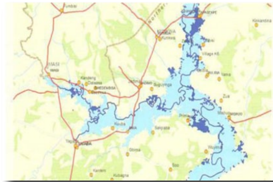
Figure 3: Flood Risk Map for the White Volta at Yagaba (see Figure 2 for position of Yagaba). Light blue are areas with very high flood risk and inundated on average every other year, while in dark blue those areas are affected in the event of major floods (every 10 to 100 years) (Source: White Volta Flood Assessment and Forecasting Report, 2012)
