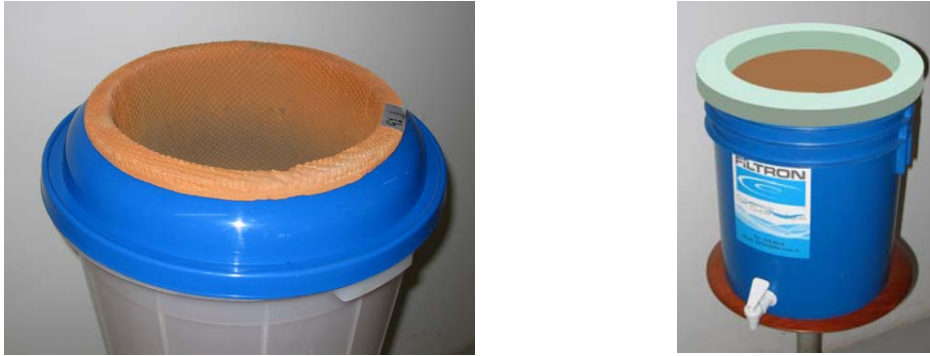
Figure 5.5 Sealing ring (a) Ghana (b) new design
