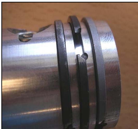
At the ring gap its worn locally
