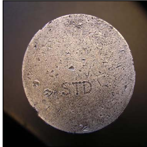
Top of damaged piston
