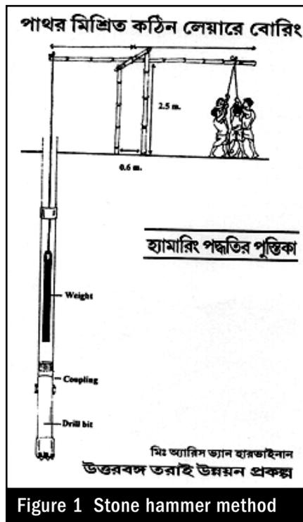
Figure 1 Stone hammer method
