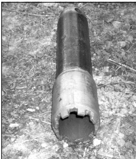
Figure 2 Hammer head or bit
