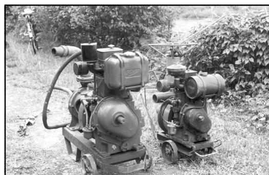
**Figure 12** The improved 2.5 hp pump set next to a common 5 hp pump set
