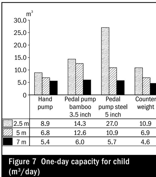
deepest level the 3.5-inch pump gave the best results for both test persons.
