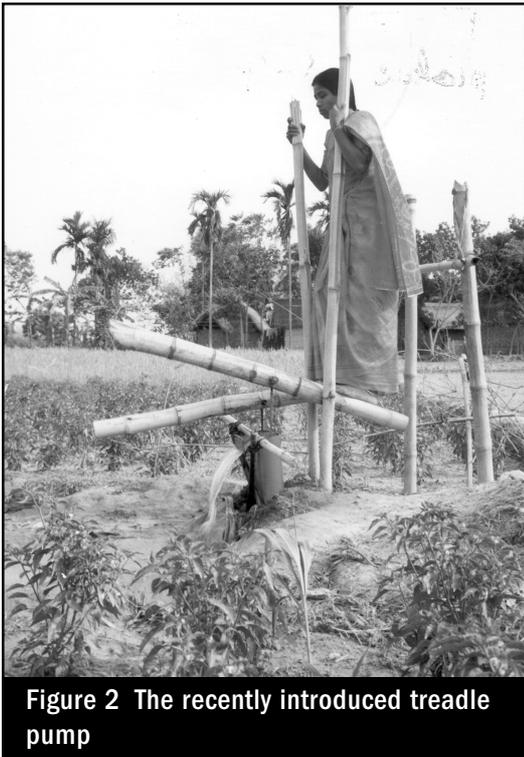
**Figure 2** The recently introduced treadle pump
