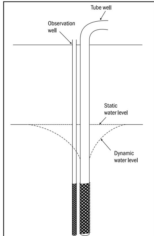
Figure 2 Draw-down at the tube well as a function of discharge
