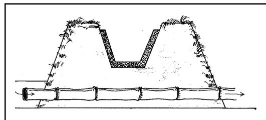
Figure 7 Use of bamboo pipes for drainage
