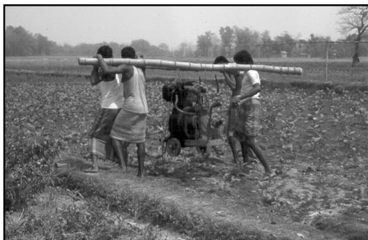
Figure 13 Moving a 5-hp pump set
