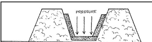
Channel bottom is pushed down and cracks occur at the joints.
