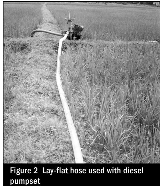
Figure 2 Lay-flat hose used with diesel pumpset
