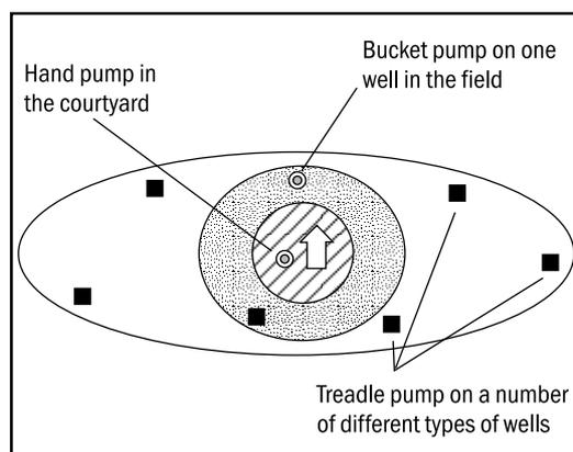
**Figure 9** Radium of action for manual pumps
