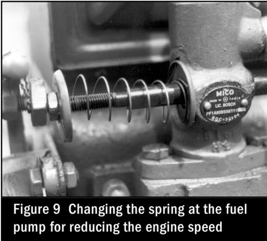
**Figure 9** Changing the spring at the fuel pump for reducing the engine speed
