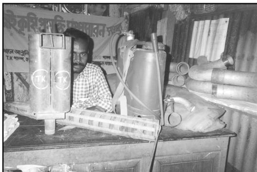
**Figure 9** Filters as used for treadle pump wells
