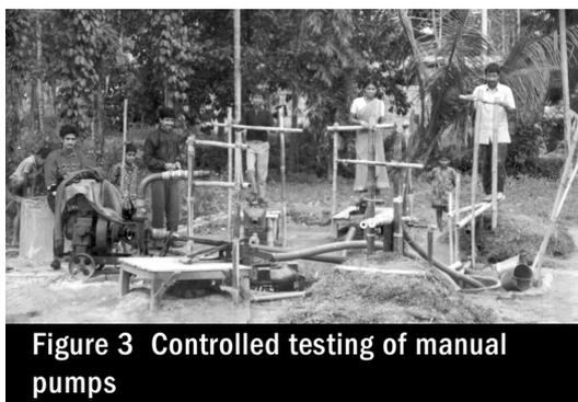
**Figure 3 Controlled testing of manual pumps**
