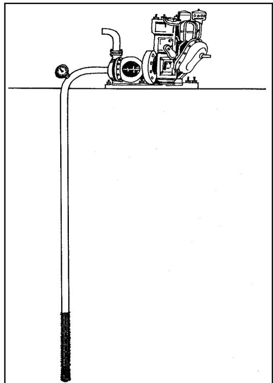
Figure 1 Pump set, well, and vacuum gauge
