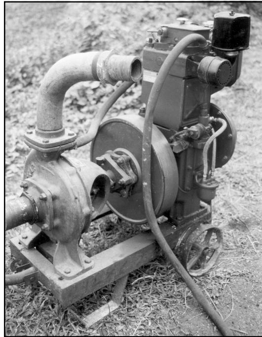
**Figure 1 Typical 5 hp/1500 RPM diesel pump, before modification**
