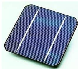
The cells may be round, square or some other shape. Each cell produces about 0,5 Volt, no matter what the size is. The amount of amperes a cell can produce does depend on its size; larger cells produce more amperes. As each cell only produces about 0,5 Volt, many cells have to be connected in series to produce a high enough voltage. Usually there are from 30 to 36 of these cells on a panel intended to charge a 12 V battery.
