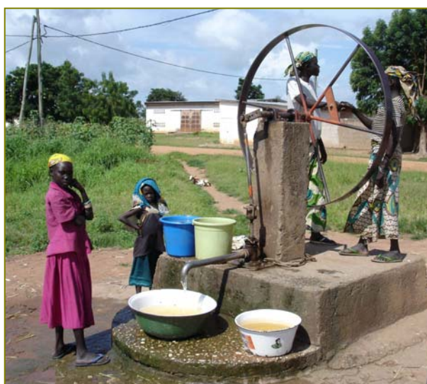
Volanta pump in Cameroon
