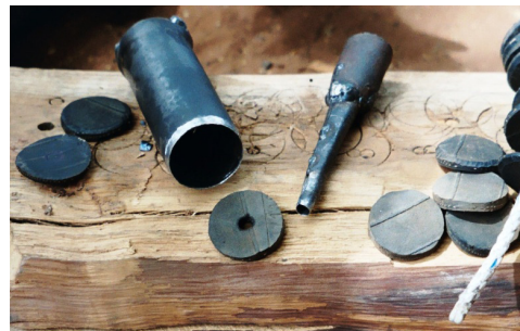
Rubber pistons made of car tire
