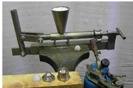
PE piston mould and extruder
