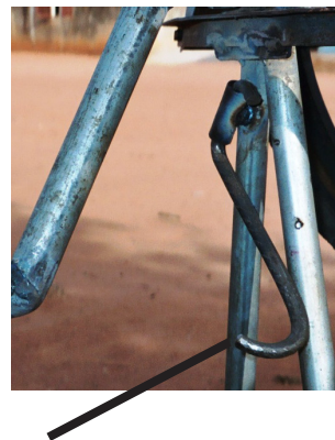
Pump lock is open during pumping
