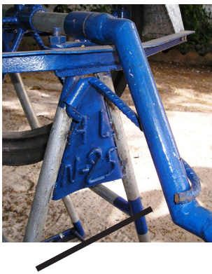
Pump lock is closed when you stop pumping
